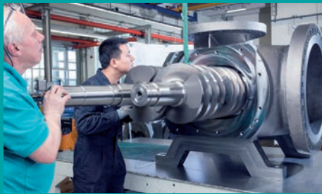
Final assembling of spindles for L4NC
