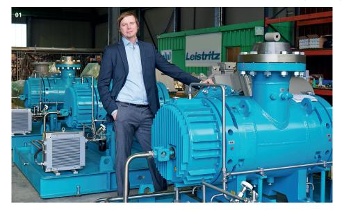
with a capacity of up to 5,000m3/h and a differential pressure of up to 100bar.
