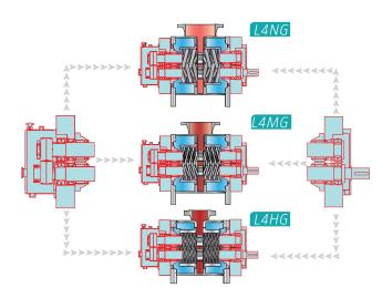
Instead of individual designs, all pumps are designed and manufactured as a modular system. While pump casings, liners and screws are still adapted to the particular operating conditions, bearing covers, bearings, timing gears and the seal components are interchangeable among pumps of different sizes.
