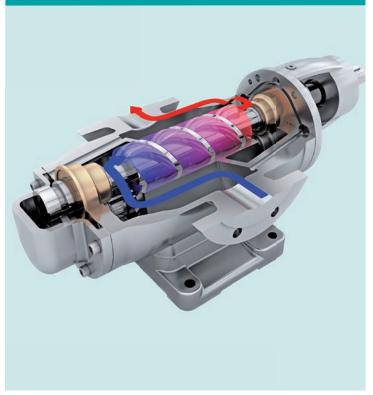
Leistritz screw pumps of the L2NG/NT series are twin screw single volute, self-priming positive displacement pumps for low pressure duty, suitable for transport of slightly abrasive and corrosive, high or low viscous fluids with poor or good lubricity.
