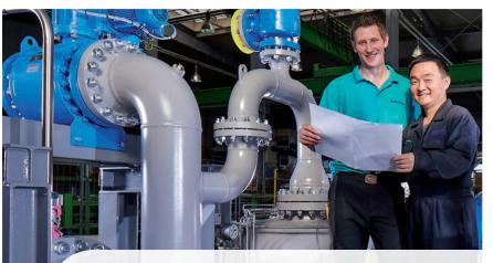
» Leistritz multiphase pumps are controlled with variable speed drives to react immediately on changing process conditions without the need of system modification and/or reinstallation. «
