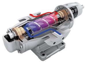
Leistritz screw pumps of the L2 series are self-priming, positive displacement pumps for a pressure range of up to 16 bar (232 psi), suitable for transporting light abrasive and corrosive, highly or low viscous fluids with poor or good lubricity.
