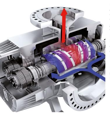
L4 Pumps are selfpriming screw pumps with two screws in double volute and hydraulically balanced design. The drive torque is transmitted from the double helix drive screw to the likewise double helix idler screw via herringbone gears.
