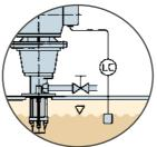
The pump is installed vertically in the tank with the discharge flange outside the tank.
